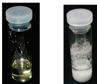
FIGURE 2. Solubility comparison of organocatalysts in CH 2 Cl 2 . The left image illustrates that 300 mg of sulfonamide 1 is soluble in 1 mL of CH 2 Cl 2 , and the right image demonstrates that 300 mg of proline is not readily soluble in 1 mL of CH 2 Cl 2 .
